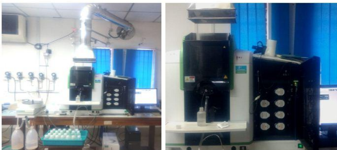
Figure 2.16: Atomic absorption spectrophotometer used in measuring heavy metals in ambient air sample.
