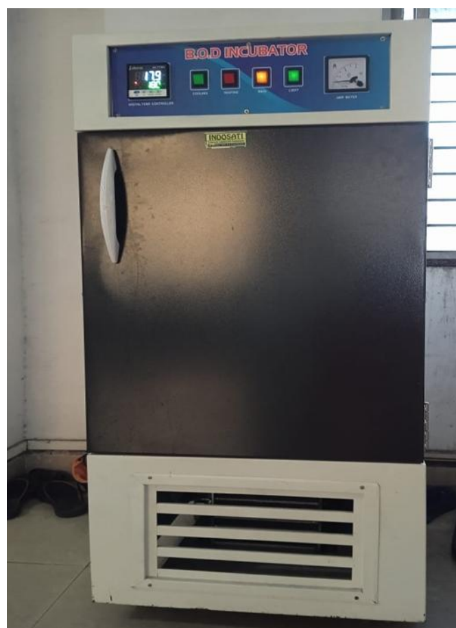
Figure 3.7: BOD incubator used in analysis.
