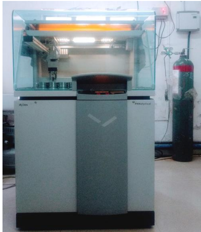
Figure 4.1: X-ray fluorescence spectrometer used for soil analysis.
