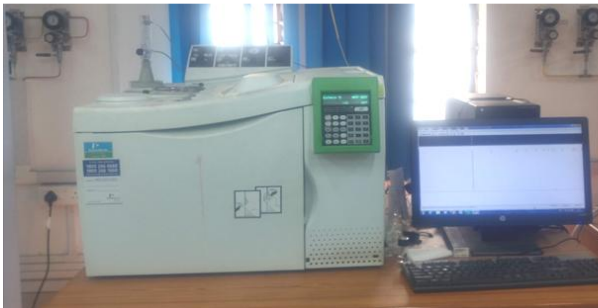
Figure 2.15: Gas Chromatography fitted with capillary column and FID detector used for PAH measurement in ambient air.
